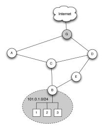
Figure 8: Router "B" is allocated the subnet 101.0.1.0/24
