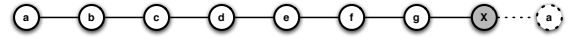
Fig. 10. Link Spoofing: The malicious router X advertises a spoofed link to router a in its TC messages, thus all routers will record the links X-a and b-a .
